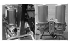
**Desiccant Air Dryer System #195 117** A regenerating inline air dryer system that eliminates moisture in the air stream to prevent air tool freeze-ups in cold climates. Internal thermostat and heating elements insure good air quality in all climates. The system can be mounted on the side of the machine or remotely for truck mount installations.
